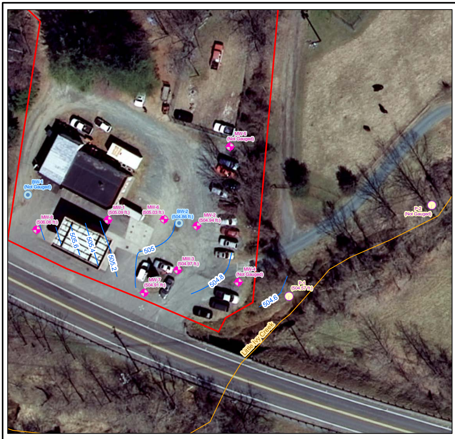
Figure 2: Site Monitoring Wells and Groundwater Elevations
